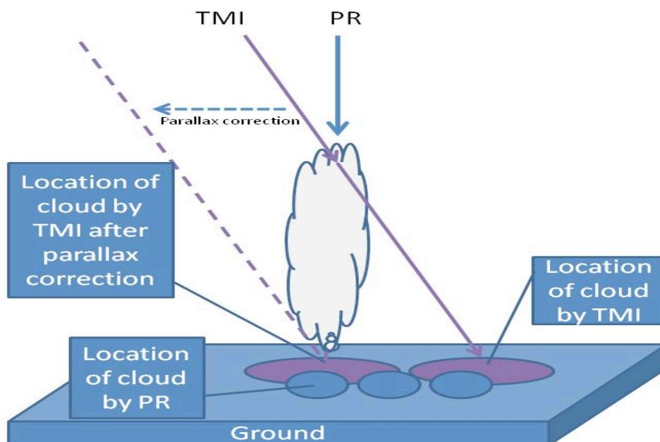
Figure 2. Schematic diagram of parallax correction.
